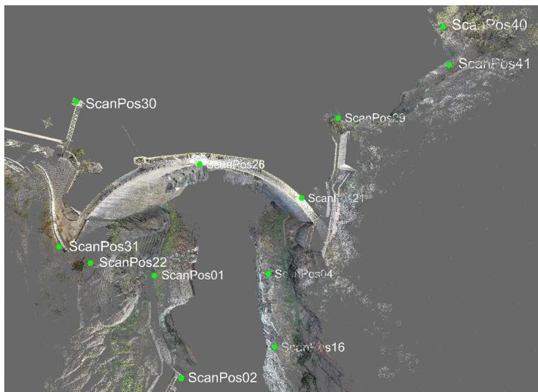
*Fig. 5 – General view of the stations using the filtered cloud of points as background*
