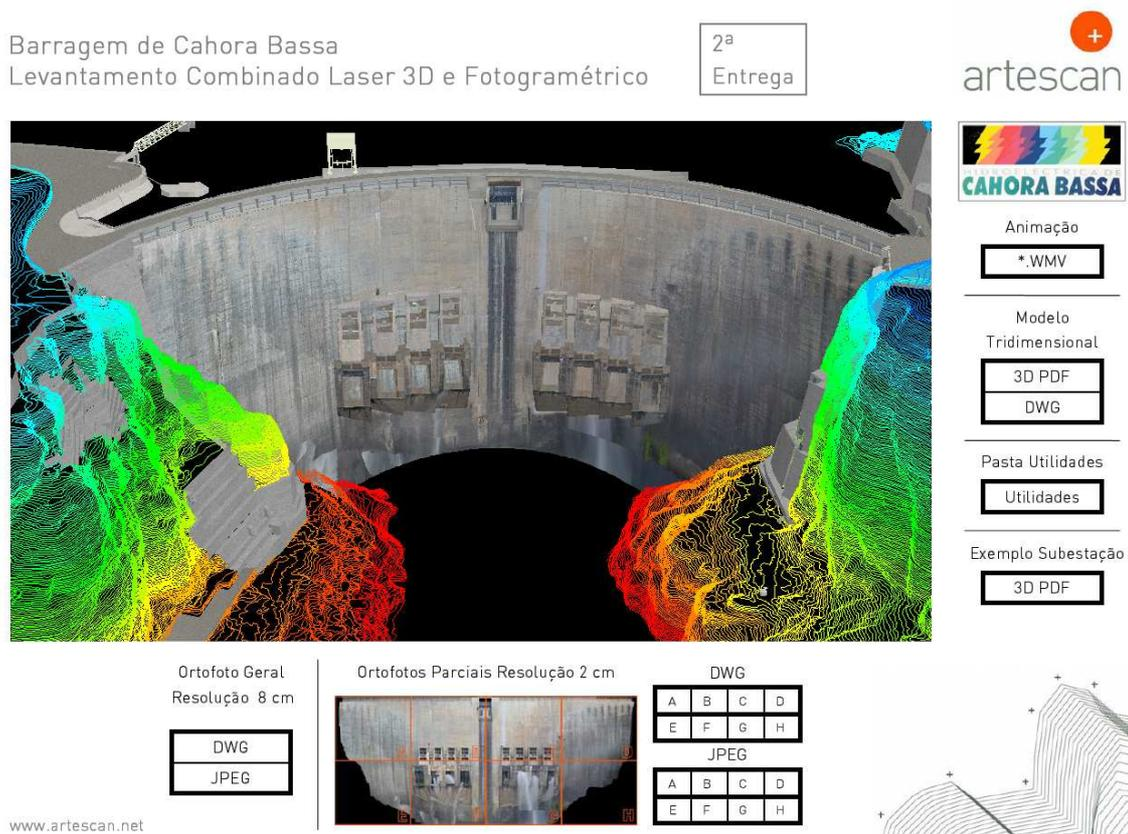
Fig. 6 – A 3D PDF file in which the main window has an interactive 3D model of the dam and envelope area and the hyperlinks to different files containing synthesized information on several electronic formats
