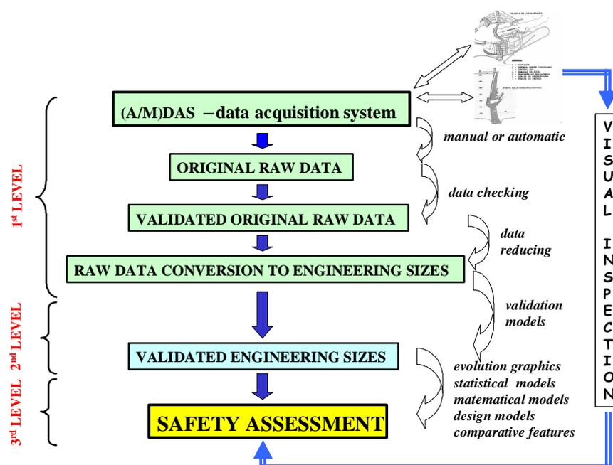
Fig. 2 – Flowchart for dam behaviour and safety control assessment
