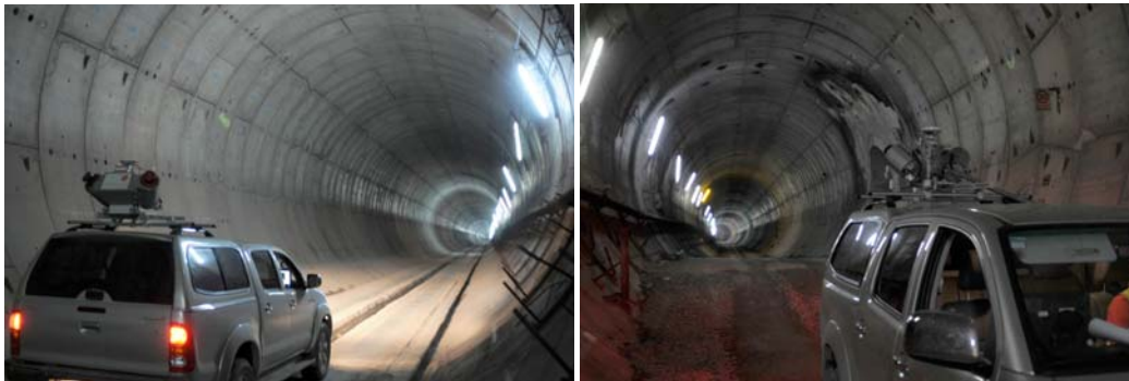
Figure 3 – RIEGL VMX-250 surveying the Pajares tunnel
