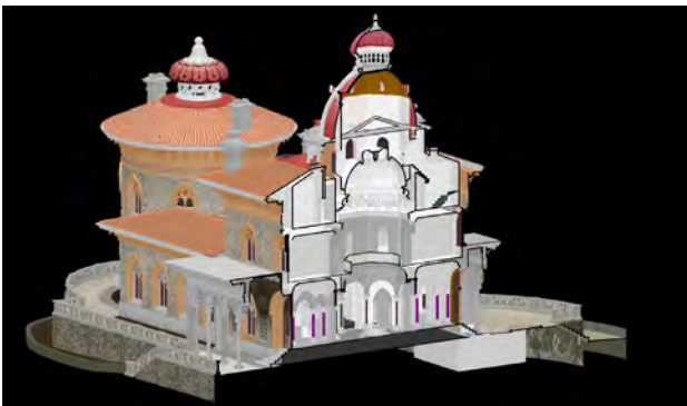
Figure 4: Cross-section cut of the Monserrate 3D model.
