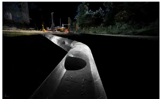
Figure 6: Site reference frames: Scanner position local reference frames on surface and underground, with transformations for both for the project reference frame. Site survey of Caneiro do Rio Tinto, Portugal.
